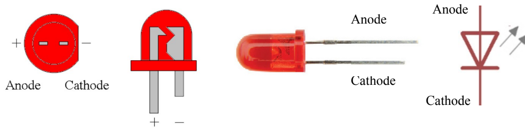
Figure 4 : Example LED IO indicators (left), LED case style / connections (right)
