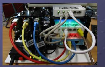
Move eth1 from Pi-2 and Pi-3 onto second switch + one patch cable between switches.
