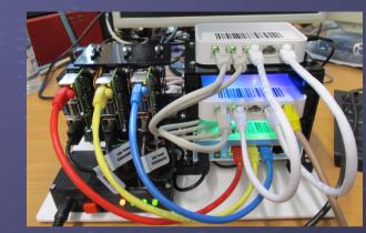
Move eth1 from Pi-2 and Pi-3 onto second switch + two patch cables between switches.
