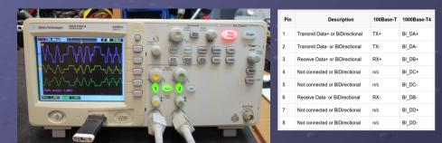
100Base-TX (Fast Ethernet) only uses two twisted pairs (4 wires) i.e. one pair for transmit, one for receive. Pins 1,2,3 and 6. (all four twisted pairs used for Gbps)
