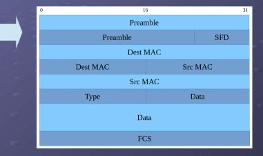
Preamble : 56 bits (7 bytes) of alternating 1' and 0's
